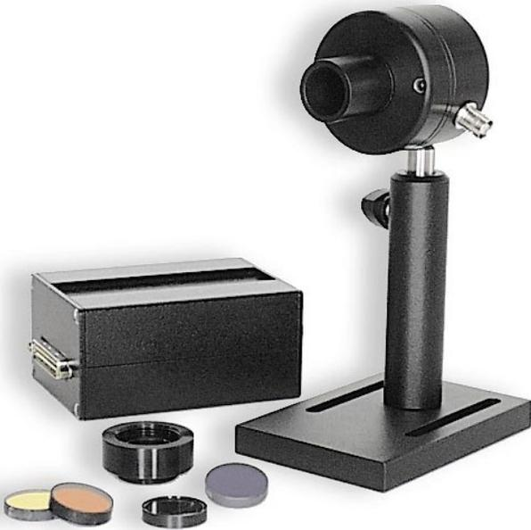
The RjP-495 Germanium Probe is designed specifically for mid-IR, pulsed energy measurements. The large size (13 mm diameter) detector is ideal for measuring total energy and fluence of eye-safe laser sources. Picojoule sensitivity, 200 Hz speed, and room temperature operation make it the probe of choice for mid-IR energy measurements.
