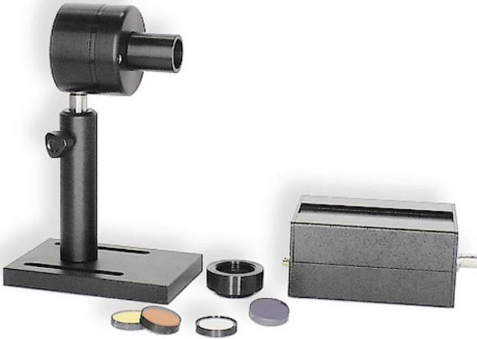
This UV-Enhanced Silicon Power probe is designed specifically for measuring low intensity, continuous wave or pulsed sources, from the near-UV to the near-IR. Picowatt sensitivity, a low noise preamplifier, and a 1 cm<sup>2</sup> active area combine for unprecedented versatility and accuracy.
