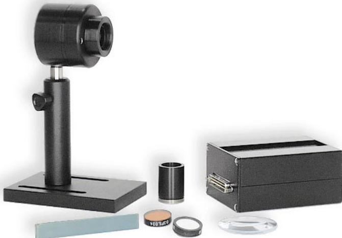
The RkP-485 is the first InGaAs Probe designed specifically for high accuracy laser power measurements. The custom InGaAs detector is 5 mm in diameter (0.2 cm<sup>2</sup> active area) - over six times larger than the typical InGaAs detector - making it very easy to use for “real world” measurements. Picowatt sensitivity and superior thermal stability make it the probe of choice for mid-IR power measurements.
